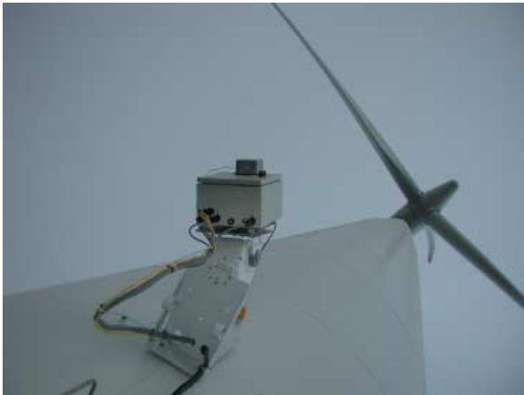
Figure 4. Photo showing the TADS mounted in the vertical mode on one of the wind turbines at the Nysted offshore wind farm, Denmark.
